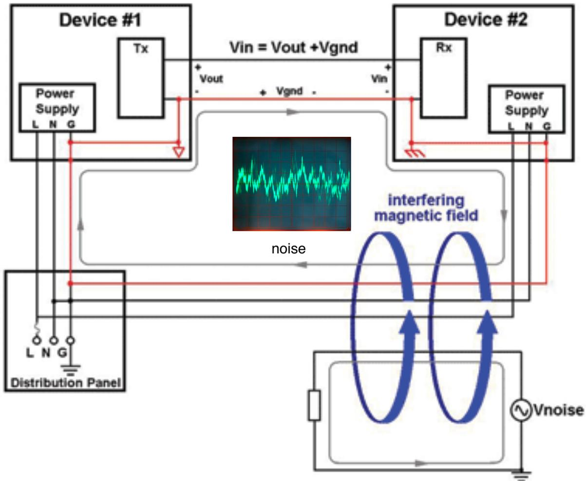
Fig. 4: Ground loop, detailed circuit.
