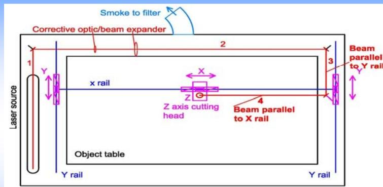
Laser generates the beam, 1,2,3,4. Mirrors 1,2,3 are fixed to the frame, mirror 4 is integral with the Y carriage, mirror Z is integral with the head.
