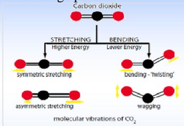
A mix of gases: CO<sub>2</sub>, He, Xe, N<sub>2</sub> fill the laser, the plasma activated by H.V. Electrodes ionize CO<sub>2</sub> to vibrate, then emit laser energy
